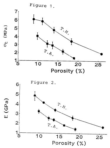
Figure 1, a plot of ot versus porosity, P(%), shows that compacts of the hydrate have a higher mechanical porosities. strength at equivalent indicating stronger bonding. The hydrate was also observed to undergo greater densification, especially at high compaction pressures. Compacts of the hydrate also have a higher Young's modulus at corresponding porosities 2), (Figure suggesting areater resistance to deformation.
